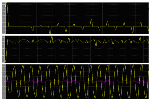
Fig. 9(f) Wave forms of load current, filter current, supply Current and supply voltage of Variable non linear load Using Fuzzy control with respect to time
